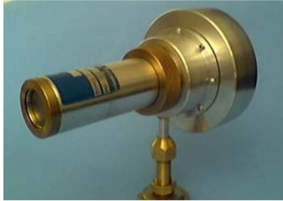
Fig. 2. Scintillation head with the bench holder.
